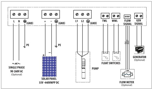
TWL = TARGET TANK WATER LEVEL WWL = WELL WATER LEVEL BOTH FLOAT SWITCHES NEED TO BE 3 WIRE TANK FILL (OPEN ON RISE, BLACK AND BLUE WIRES) GENERATOR CONTACT WILL CLOSE IF NO AC AND DC DROPS BELOW 90V.
