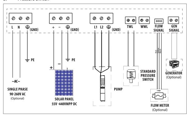
FOR PRESSURE SWITCH CONTROL, USE A NORMAL PRESSURE SWITCH OF SUITABLE RANGE – SWITCH OPENS ON PRESSURE RISE
