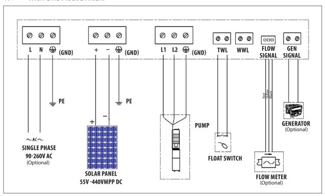
TWL = TARGET TANK WATER LEVEL WWL = WELL WATER LEVEL USE 3 WIRE FLOAT SWITCHES WIRED FOR TANK FILL (OPEN ON RISE - BLACK AND BLUE WIRES)
